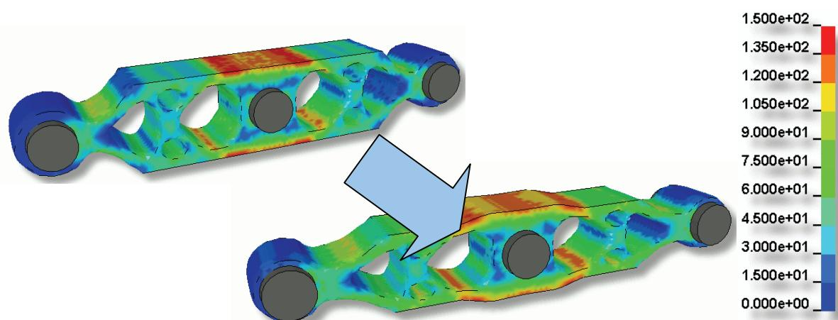
*Figure 5: Shape Optimisation Results (Von-Mises Stress)*
