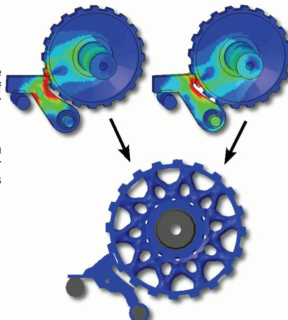
*Figure 3: Implicit LS-DYNA Topology Optimisation of Gear Design Results*
