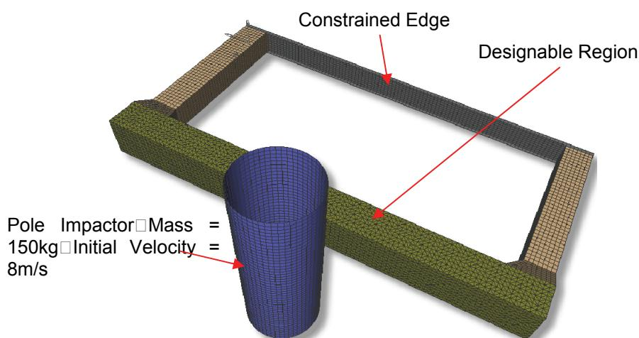
Figure 6: Pole Impact Design Space Model
