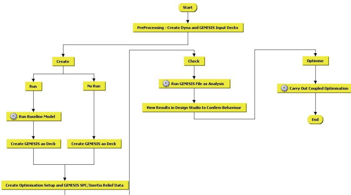
Figure 1: Coupled Optimisation Procedure
