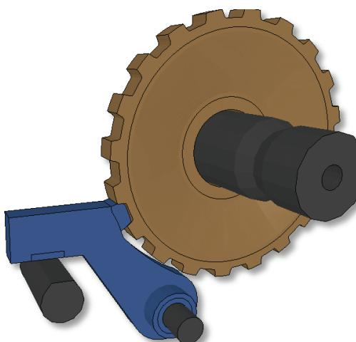
*Figure 2: Implicit LS-DYNA Topology Optimisation of Gear Design Model*
