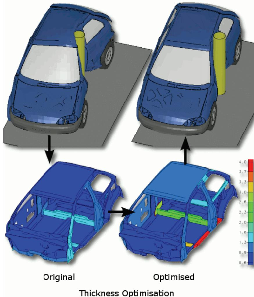
*Figure 9: Sizing Optimisation Results of Vehicle Pole Impact & Body Torsion*
