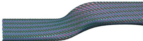
PAM-RTM for infiltration simulation (TRIA – mesh)
