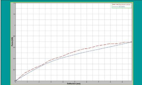
Figure 5. Load-Deflection Curve for Simulation and Experiment [Ref 5]
