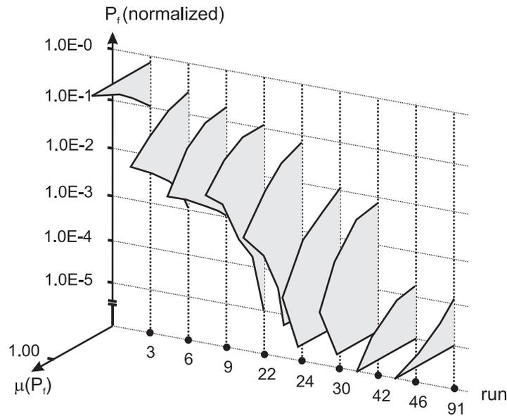
Figure 6: Fuzzy failure probabilities in selected optimization states
