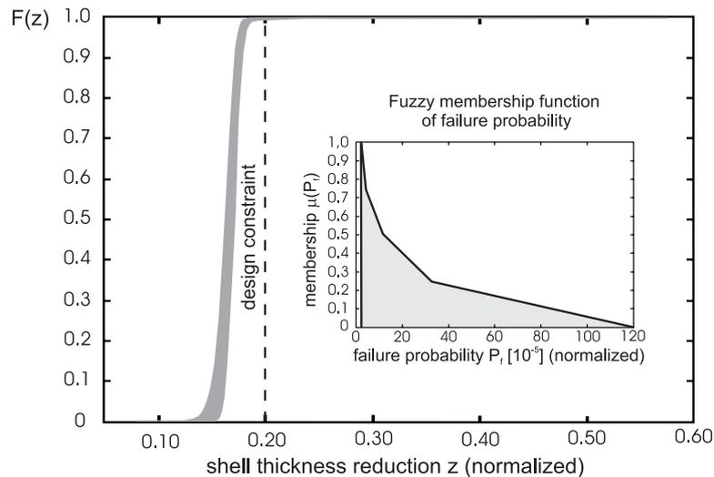
Figure 7: Result of optimal design; fuzzy cumulative distribution function and fuzzy failure probability
