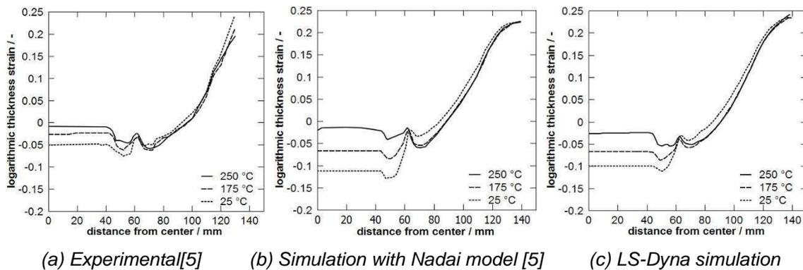
Figure 2: Experimentally and numerically determined thickness distributions
