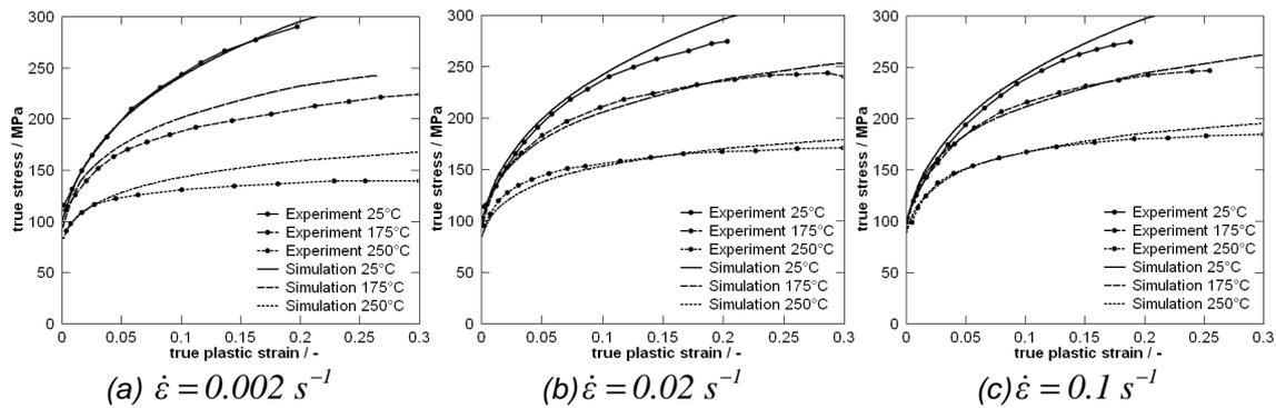
Figure 1: Experimental [5] and LS-Dyna simulation results of the uniaxial tension test
