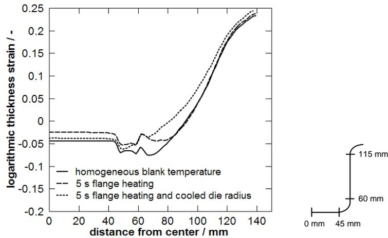
Figure 3: Thickness distribution results for different process layouts at 250 °C flange temperature and 20 mm/s punch velocity
