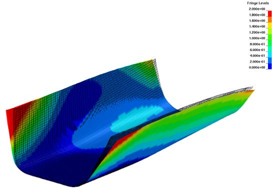
Figure 5: Result of springback simulation (displacement from intended geometry evaluated)
