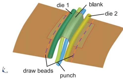
Figure 4: Model of deep drawing process
