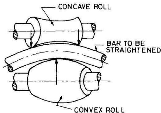
Figure 2: Bar straightening in a cross roll straightening machine (from [2]).
