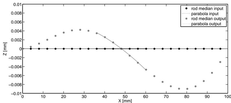
Figure 10: In- and output rod curvatures in the XZ plane.
