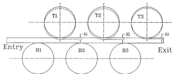
Figure 1: Schematic straightening of railway rails (from [1]).
