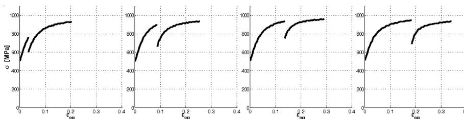
Figure 7: Different plastic pre-straining in compression with a subsequent tension loading
