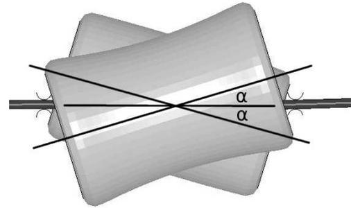
Figure 4: The angle  $\alpha$  between the rolls and the bar.
