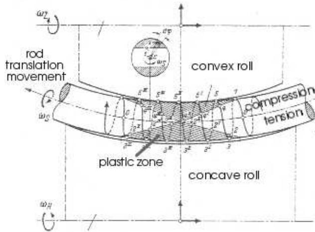
Figure 3: The plastic zone in the bent rod is propagated along a helix (from [5], modified).
