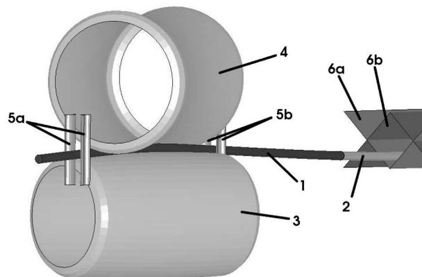
Figure 6: The different parts of the model. The rod (part No 1) moves from right to left as the rolls (parts No 3 and 4) rotate.
