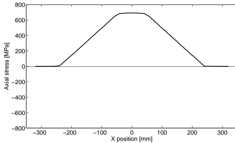
Figure 5: Axial stress of the elements in contact with the concave roll during the closing of the rolls (simple three points bending simulation) as a function of their position along the bar axis.
