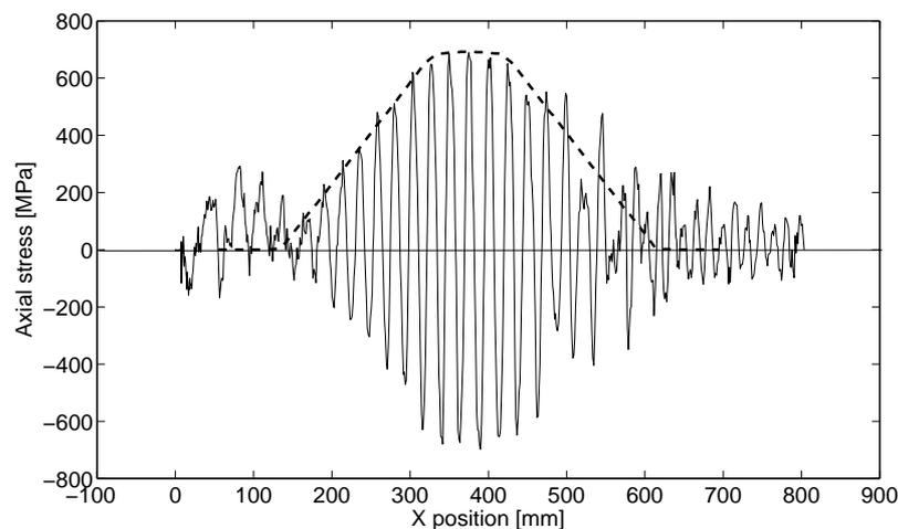
Figure 8: Axial stress acting on an element on the outer layer of the rod as a function of its position between the rolls. The stress envelope corresponds to the stress distribution obtained in bending.
