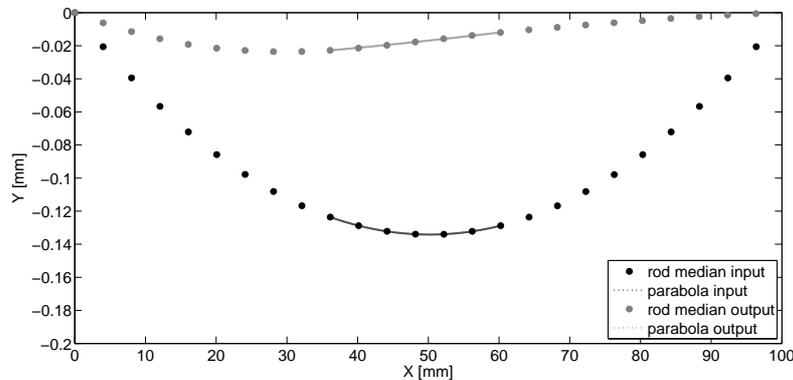
Figure 9: Parabola fitted to in- and output nodes from the median line of the rod in the XY plane.
