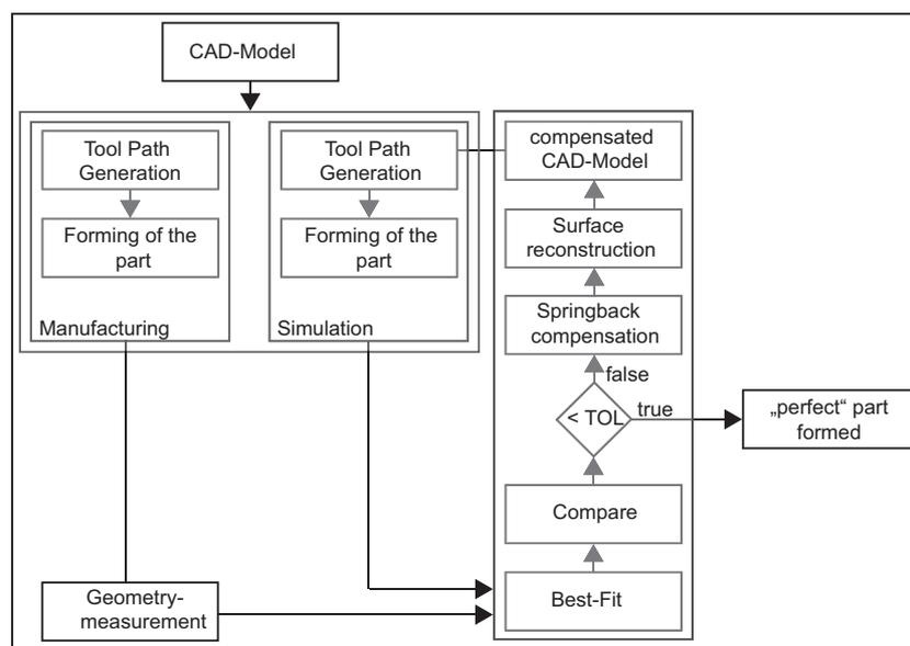
Figure 1: Springback Compensation procedure
