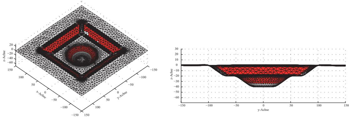
Figure 5: White sub areas detected by region growing which allow for further movement
