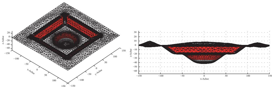
Figure 6: Final result after global and local springback procedure.
