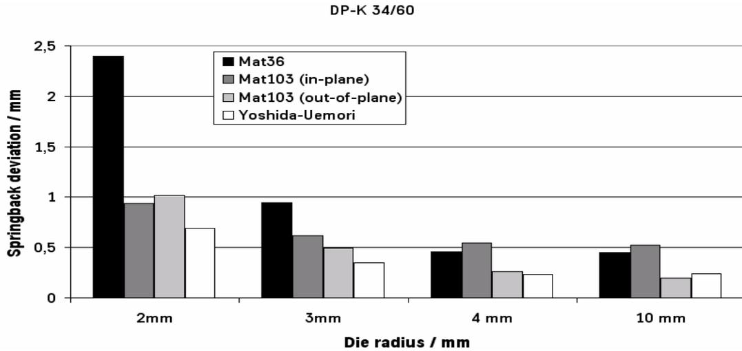
Fig. 9: FEM springback prediction errors for DP-K 34/60
