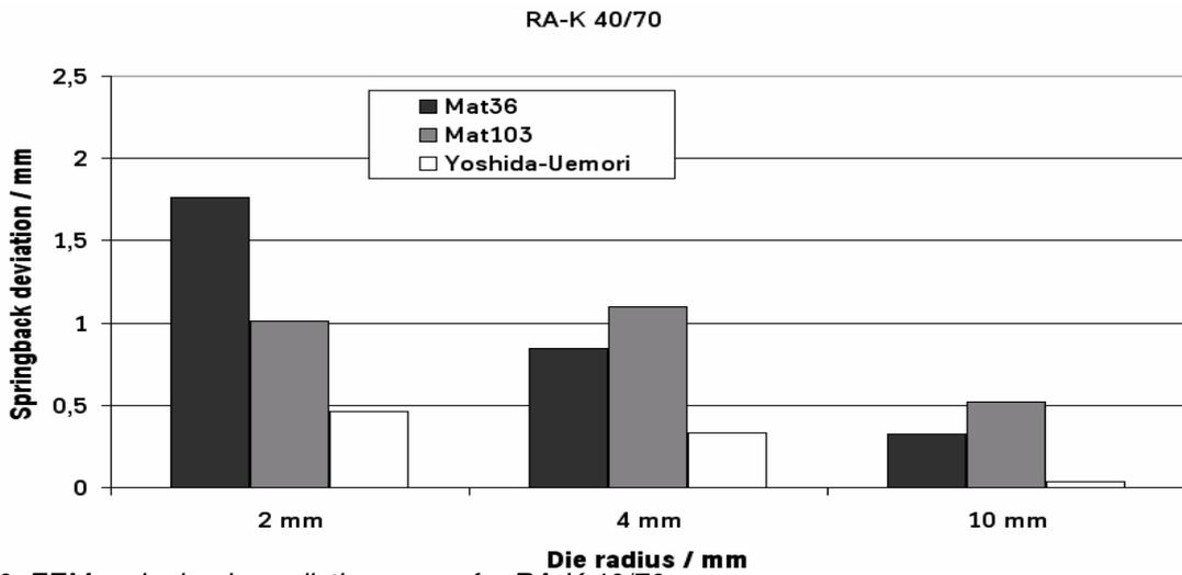
Fig. 10: FEM springback prediction errors for RA-K 40/70
