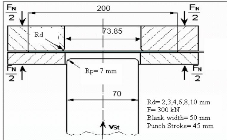
Fig. 7: Experimental set-up for the channel draw test
