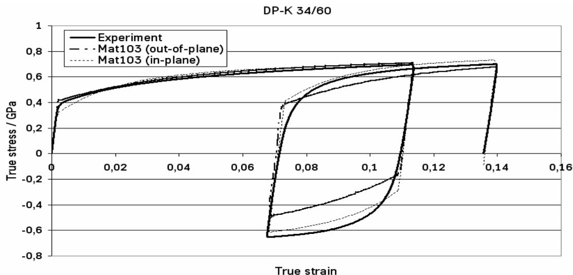
Fig. 6: Hardening characterization of DP-K 34/60 via two different kinds of tests
