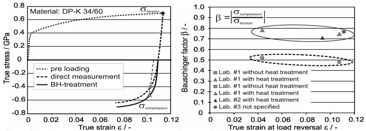
Fig. 1: Bake hardening effect in tension-compression tests [4]
