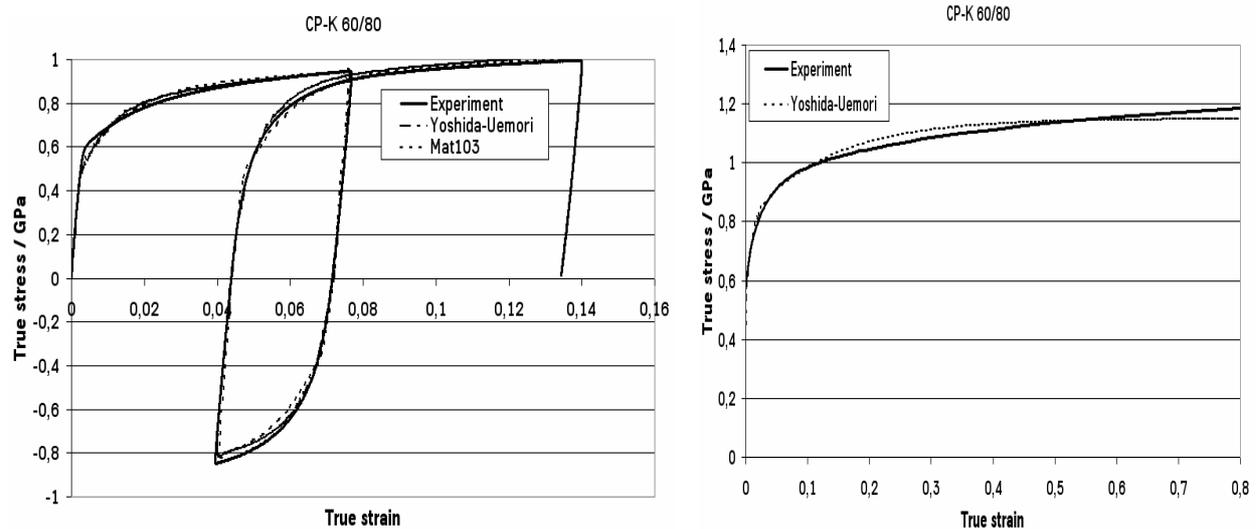
Fig. 4: Material model calibration of Yoshida-Uemori and Mat103 for CP-K 60/80
