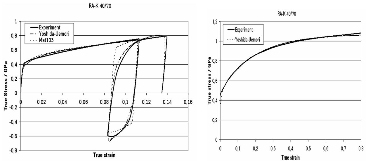
Fig. 3: Material model calibration of Yoshida-Uemori and Mat103 for RA-K 40/70
