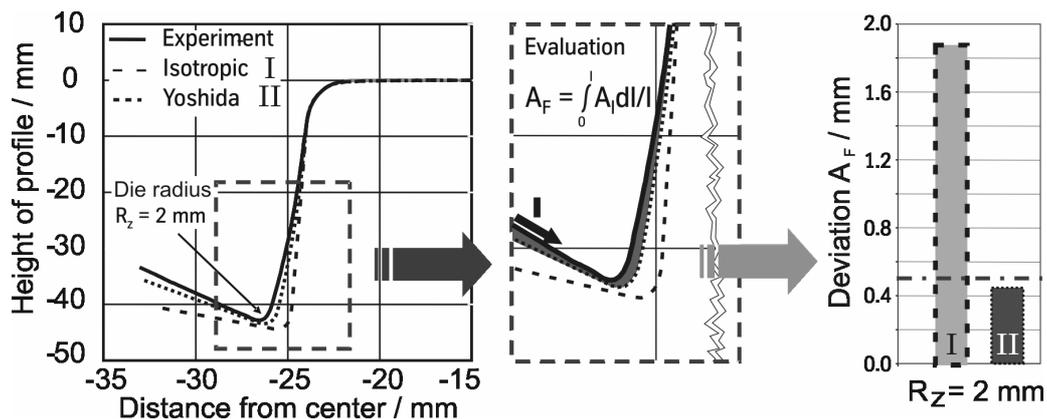
Fig. 8: Evaluation parameter for deviations compared with experimental results [4]
