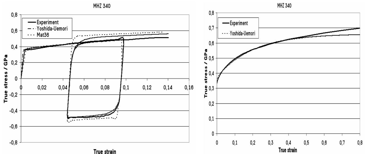
Fig. 5: Material model calibration of Yoshida-Uemori for MHZ 340
