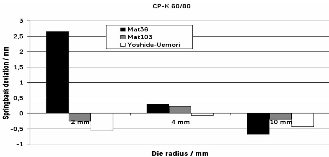
Fig. 11: FEM springback prediction errors for CP-K 60/80
