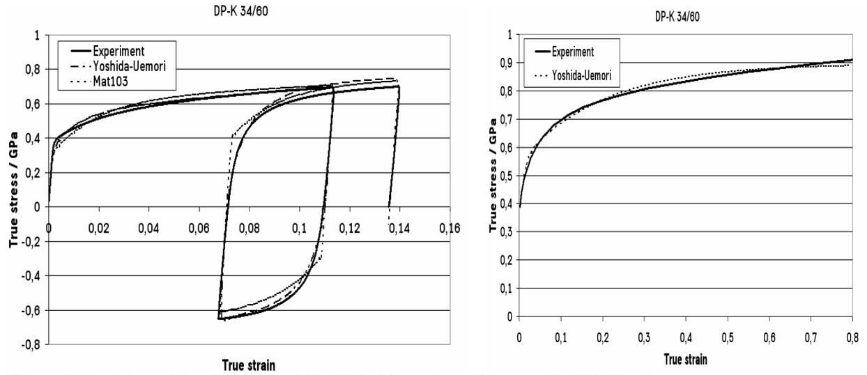
Fig. 2: Material model calibration of Yoshida-Uemori and Mat103 for DP-K 34/60
