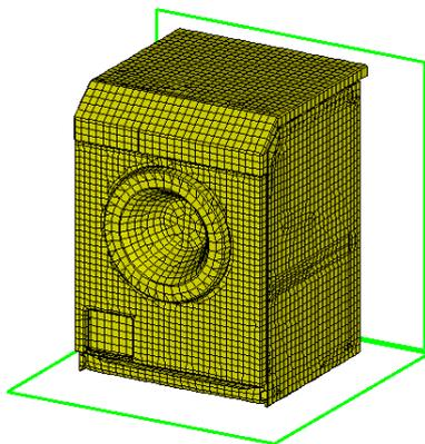
Figure 12: MBD/FEM/BEM model of a washing machine
