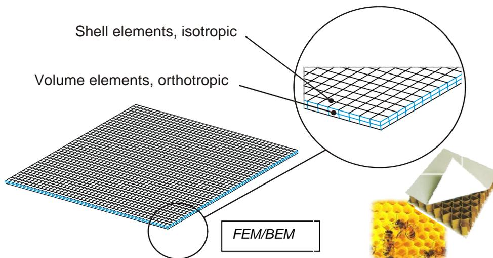
Figure 5: Structural finite element model of a honeycomb plate
