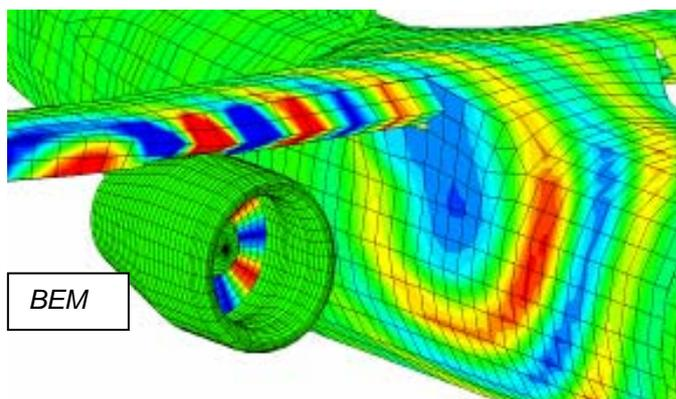
Figure 2: Sound pressure distribution at the surface of an aircraft section
