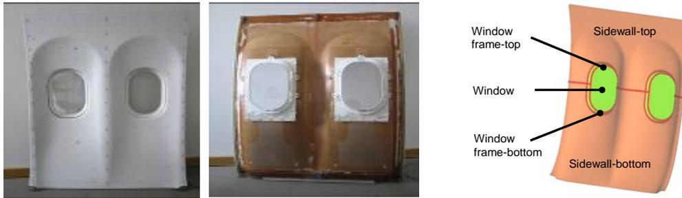
Figure 8: Side wall panel of an aircraft and its SEA model
