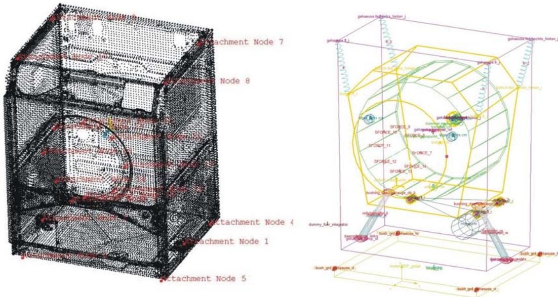
Figure 11: Integration of the elastic body structure in the MBD simulation
