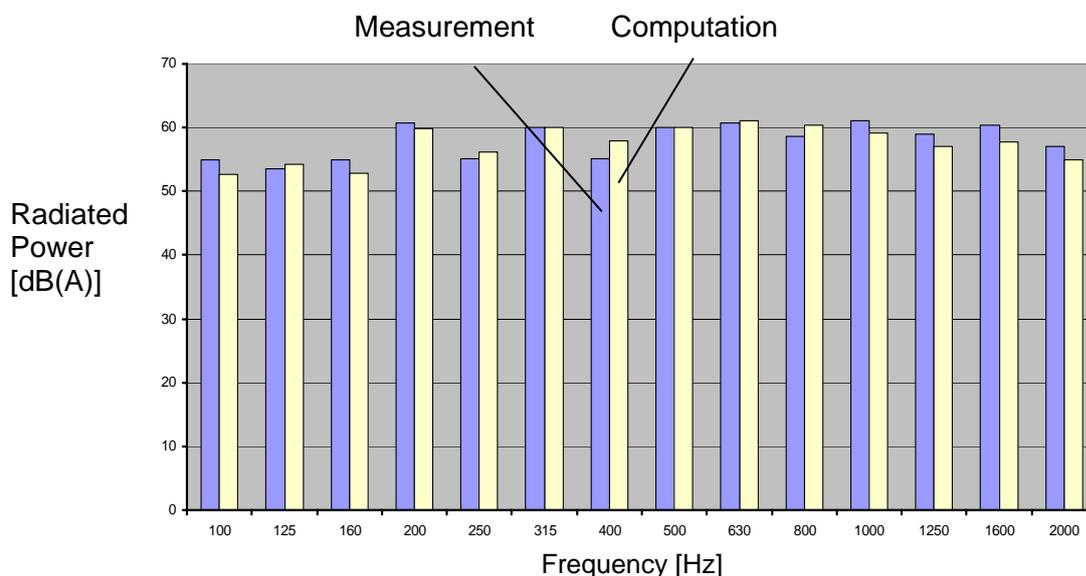
Figure 13: Comparison of measured and computed sound power
