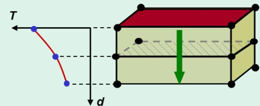
***Accuracy of forming simulations strongly depends on the consideration of temperature dependent viscoplasticity***
