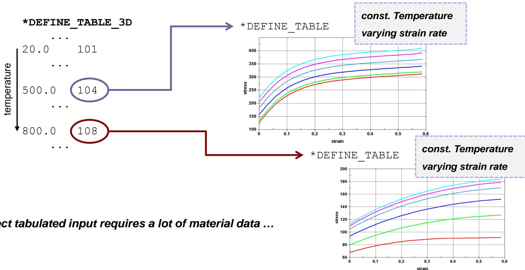
***Temperature dependent material properties require an accurate calculation of the inhomogeneous blank temperature during the forming operation***
