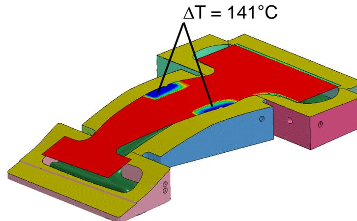
**Tool surface temperature directly affects the heat flux from blank to the die**
