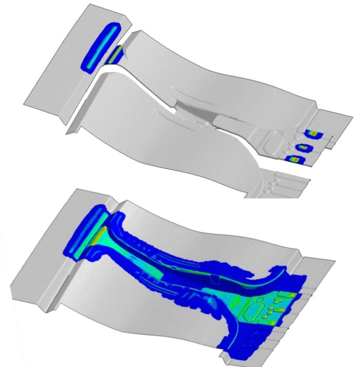
**Tool surface temperature directly affects the heat flux from blank to the die**
