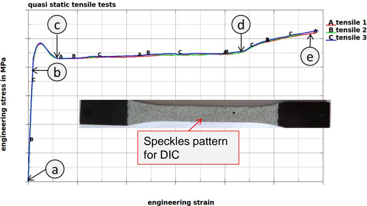
Deformation and strain at different stages
