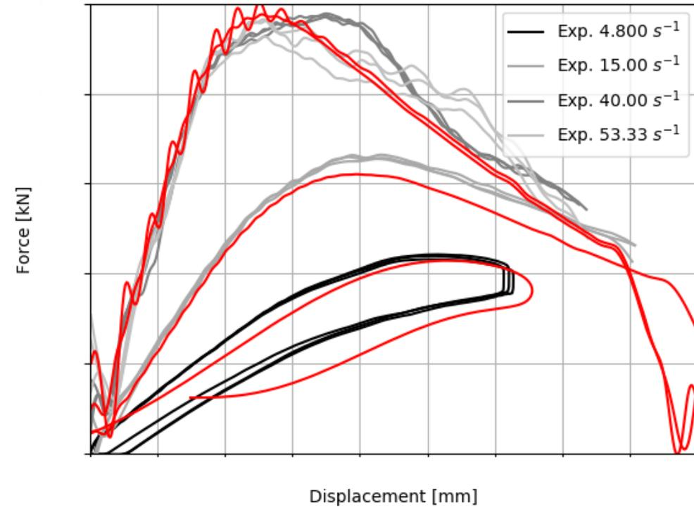
The failure modeling is able to predict the fading conduct of the strain at failure while causing no failure at bending tests as observed in the experiments performed with the pendulum.
