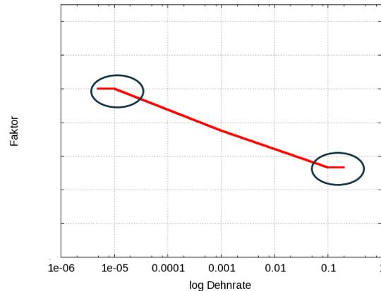
Dynamic tensile tests on polymers usually show that the strain at failure is getting shorter as the specimen is pulled faster.
