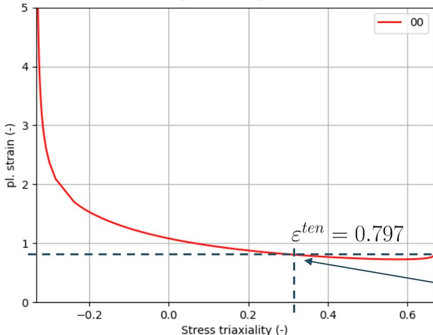
The “local” strain at break observed in the DIC measurement is around 0.9. After few iterations, a value of 0.797 in combination with the introduced Cockcroft & Latham criterion provided a satisfactory correlation with the eng. stress-strain curve:
