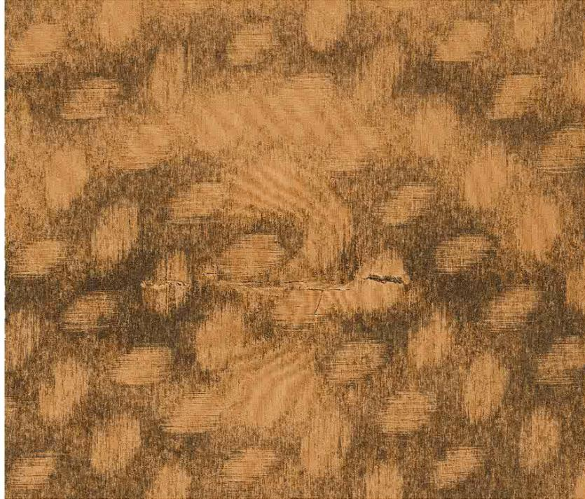
Plate consisting of 12 layer carbon fabric and rubber layer in the middle: damage after impact loading
