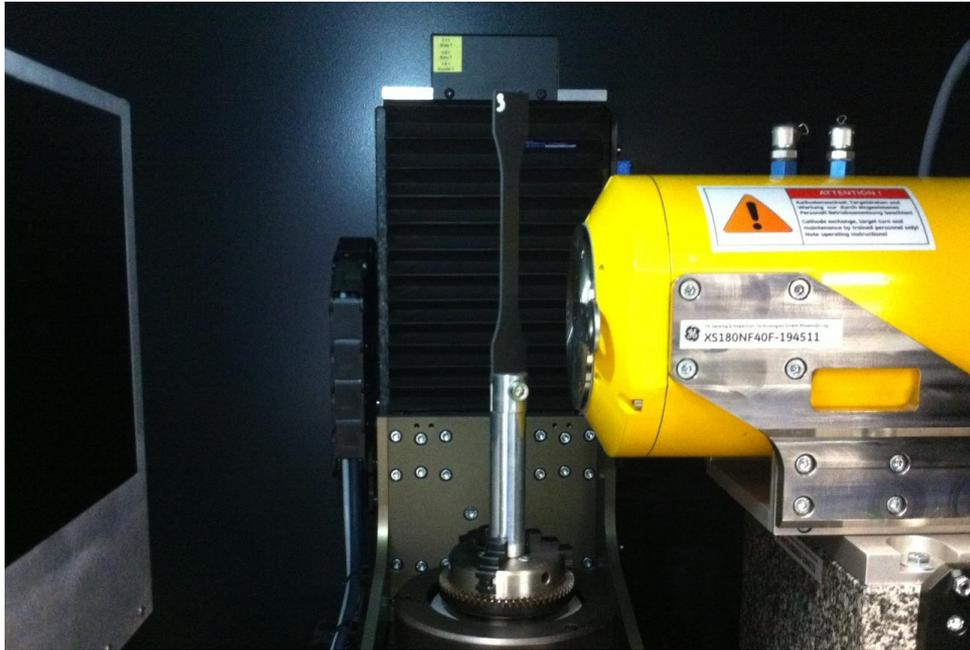
tensile specimen of short fibre reinforced plastic
