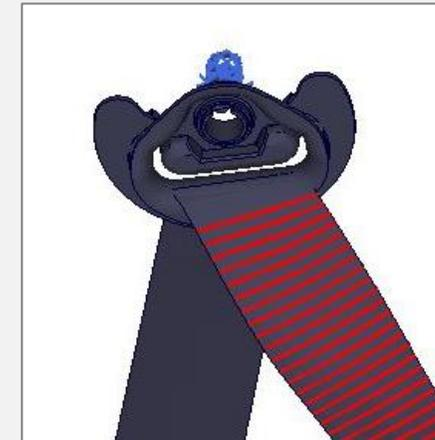
**(1) Elasto-plastic beam elements** form a plastic hinge. Verification using the 'bending line' of the webbing & loadcurves of the component tests.
