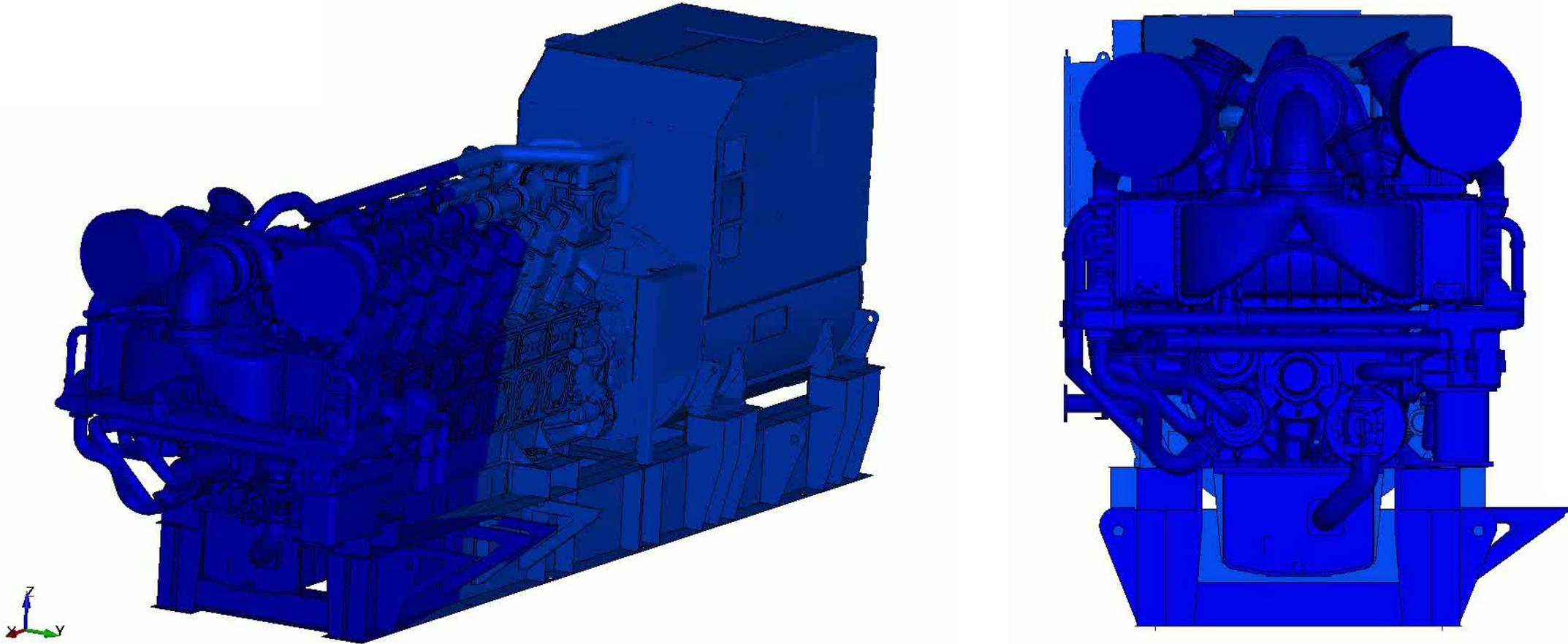
Deformation response of the system for 750ms for the shock impulse given for 50ms
