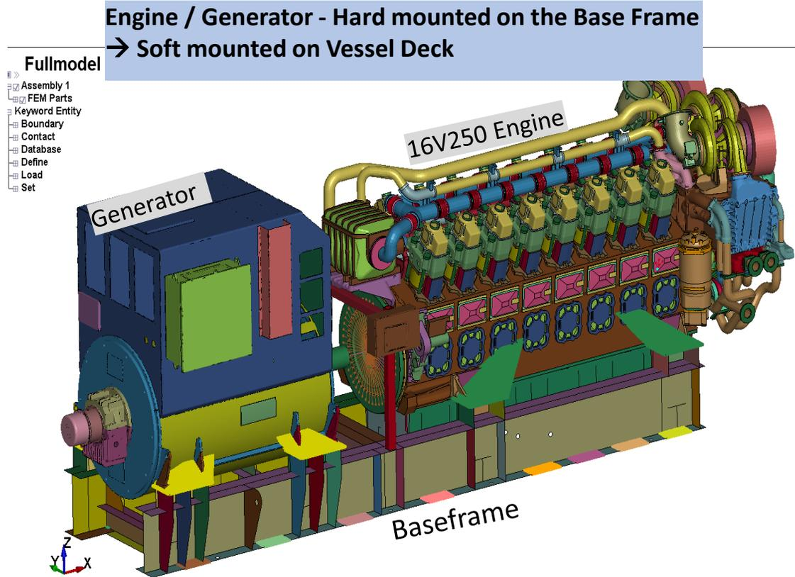
Stage 2 : Full 3D Engine and alternator simulated using SOLID elements
