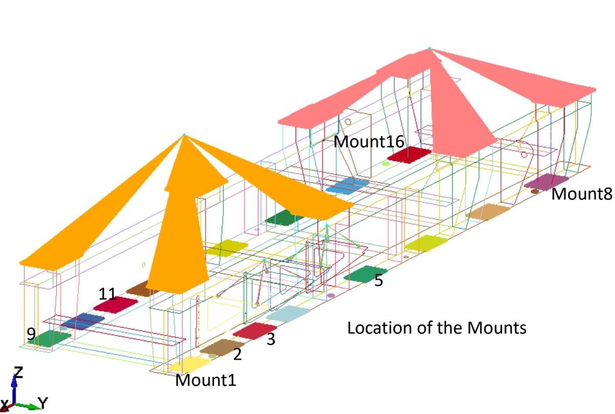
Stage 1 : Simplified model with engine and alternator as Inertia elements
