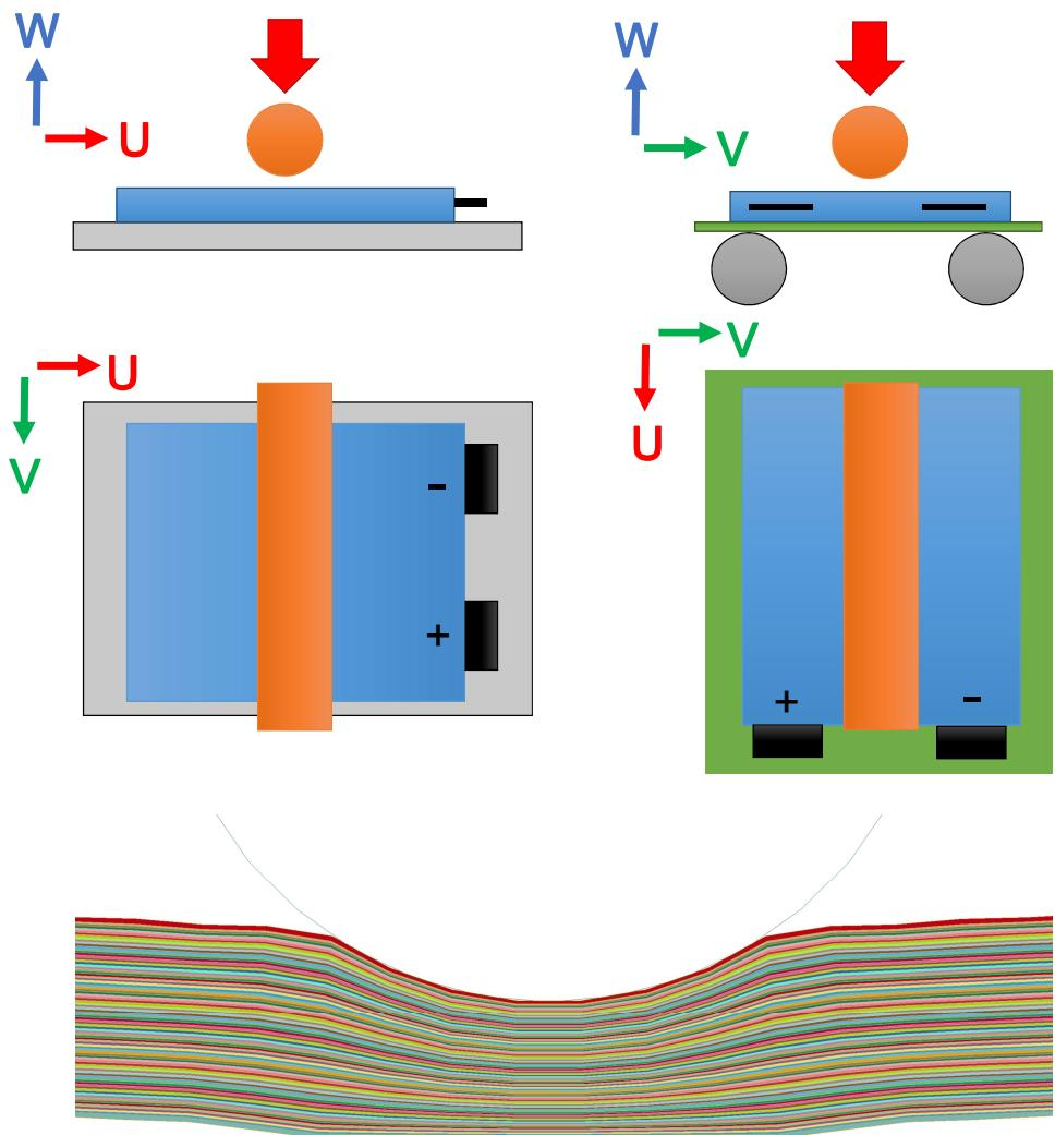
Due \*SECTION\_SOLID\_ELFORM 9 the time step size is constant: 1.33E-5ms
