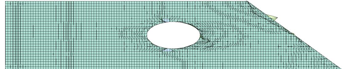
Reference Mesh Transformed to New Mesh
