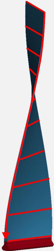
1. Description of several cross-sections of blade (by 2<sup>nd</sup>-order B-spline interpolation between given points)
