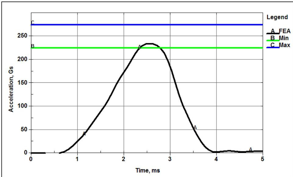
Figure 3 – 2.72m/s Calibration Test, Resultant Acceleration
