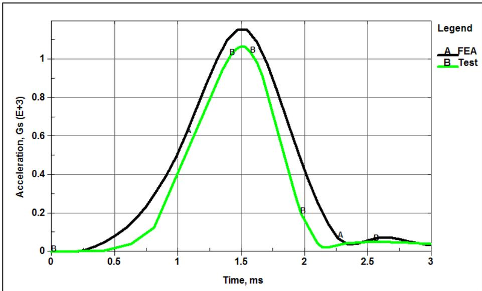
Figure 5 – 6.71m/s Calibration Test, Resultant Acceleration
