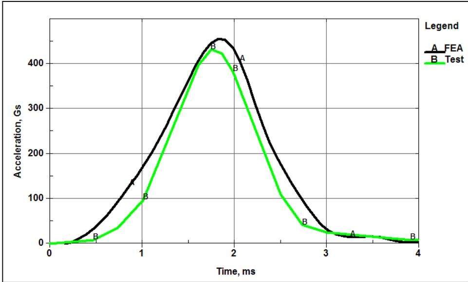
Figure 4 – 4.00m/s Calibration Test, Resultant Acceleration
