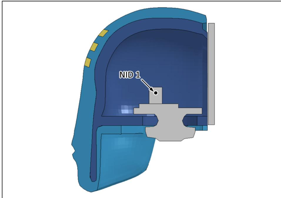
Figure 6 – CG / Accelerometer Location
