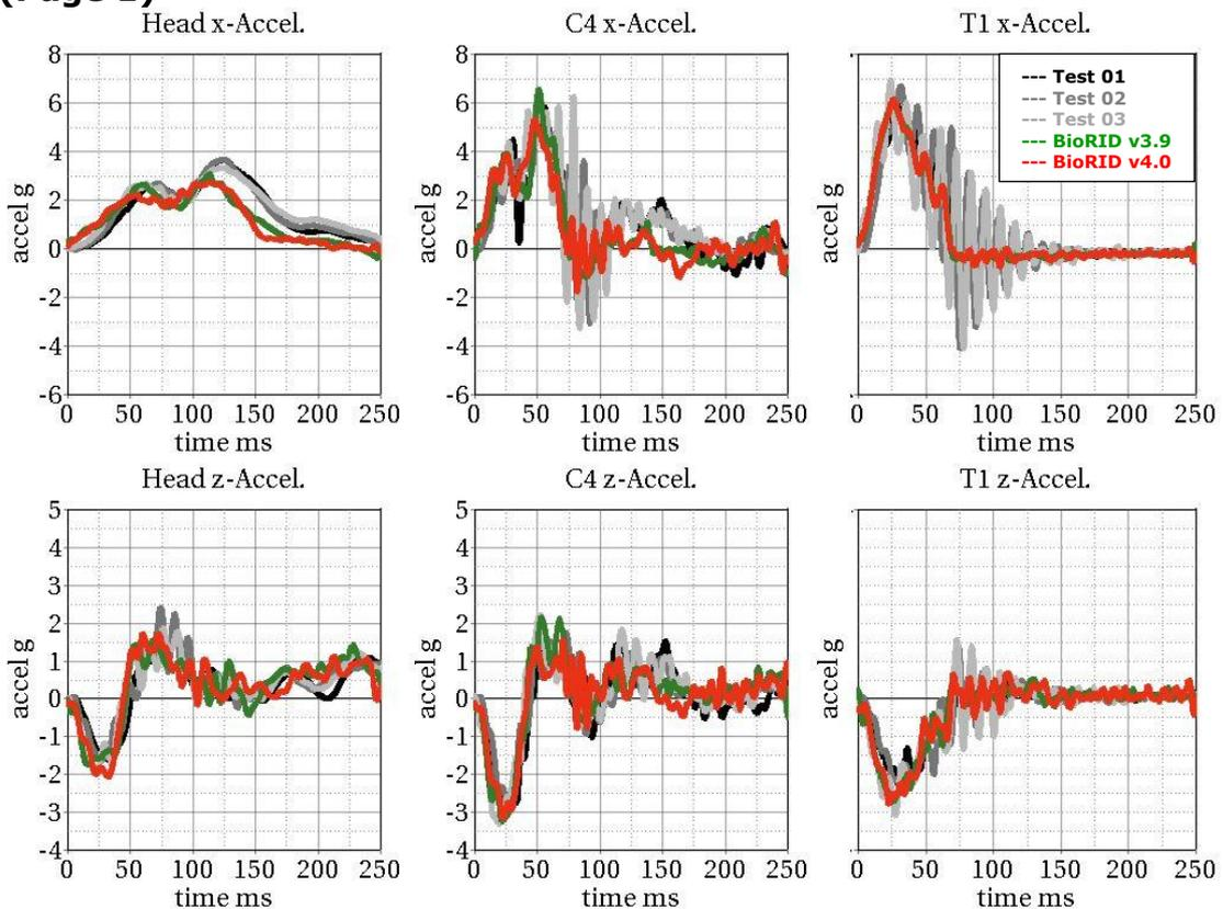
**Spine fixed up to T1 without damper/with muscle substitute springs
