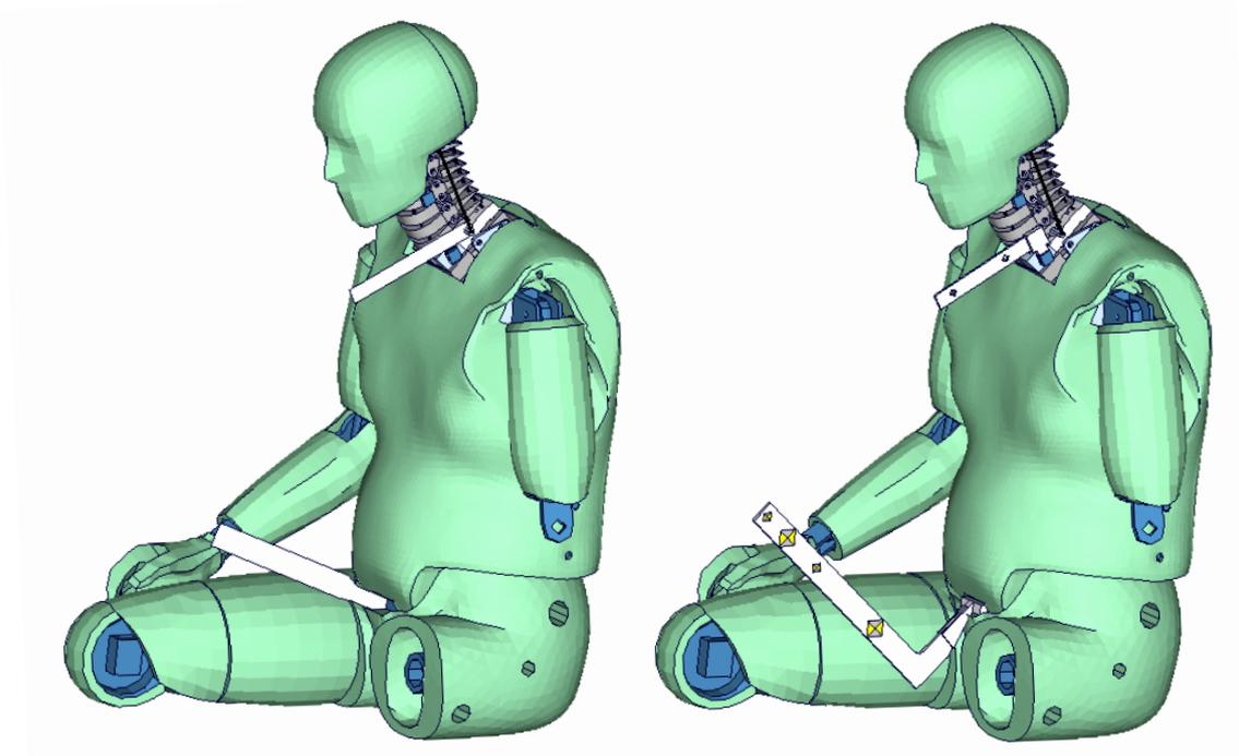
**Figure 15:** pelvis position indicator of v3.0 and v3.1 of BioRID-2
