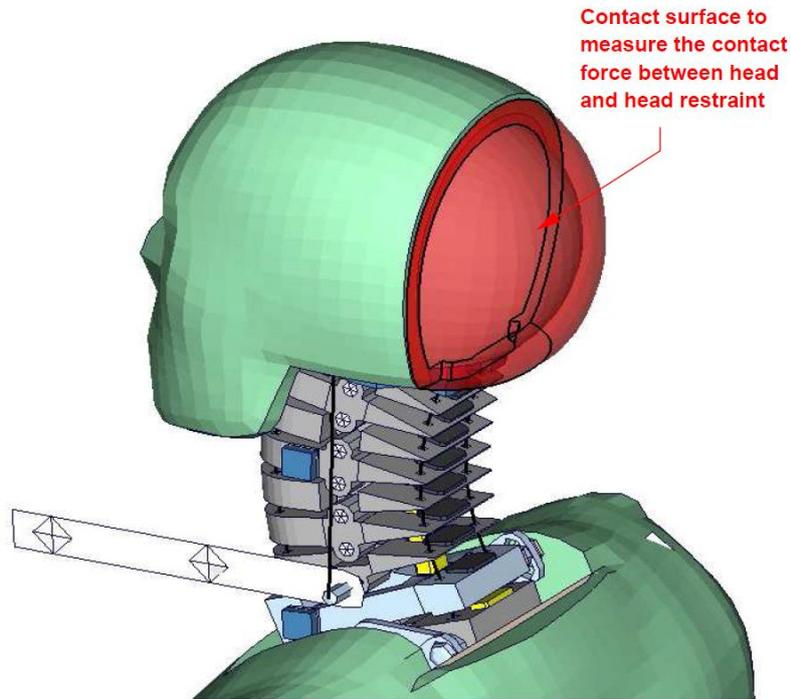
**Figure 7:** Shells to extract force on the Head.
