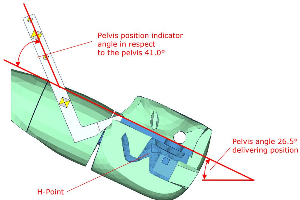
**Figure 9:** Location of H-Point and initial pelvis angle.
