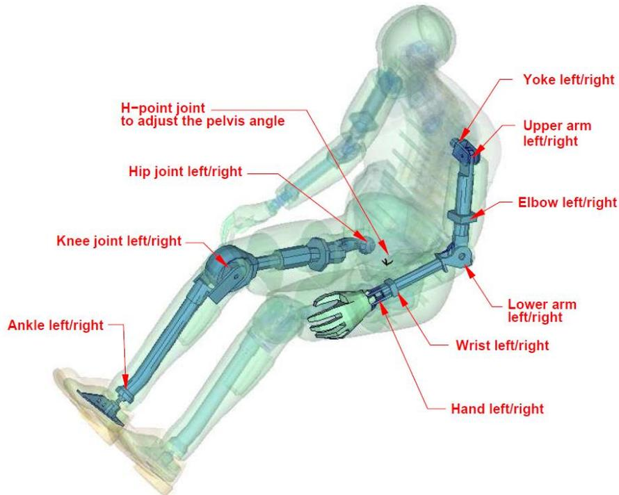
**Figure 8:** Cut through the model with joints.
