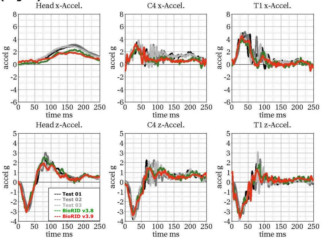
**Spine fixed up to T8 with damper/with muscle substitute springs (Page 2)**
