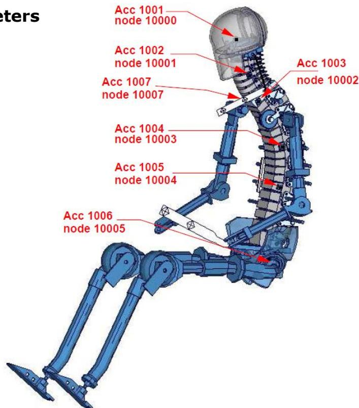
**Figure 1:** Location of accelerometers and history nodes.
