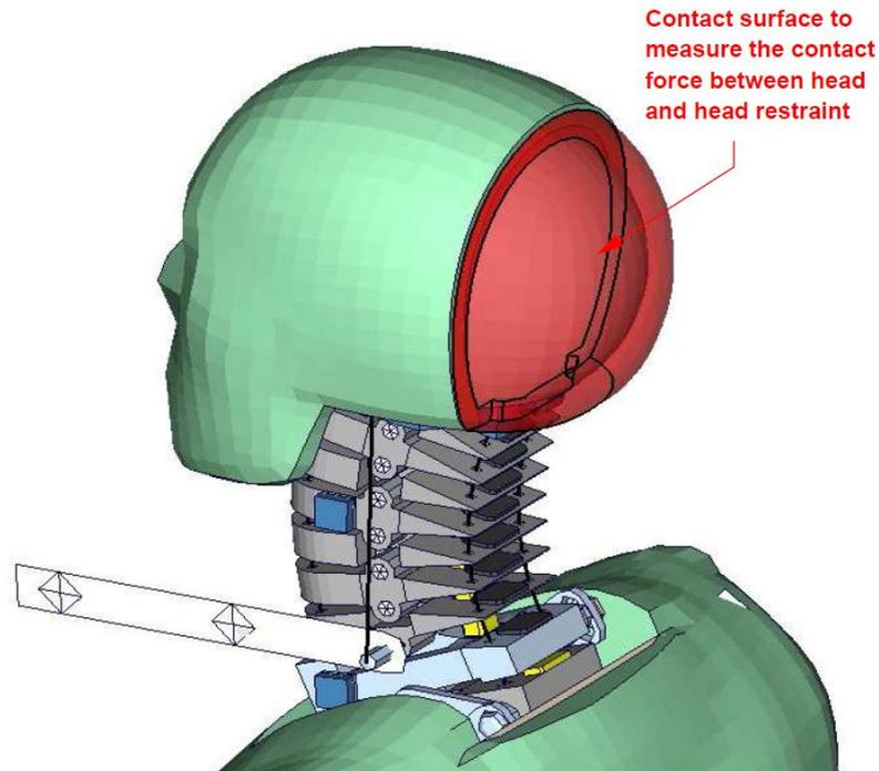
**Figure 7:** Shells to extract force on the Head.
