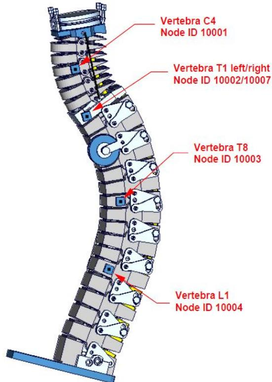
**Figure 3:** Node for extracting spine acceleration.
