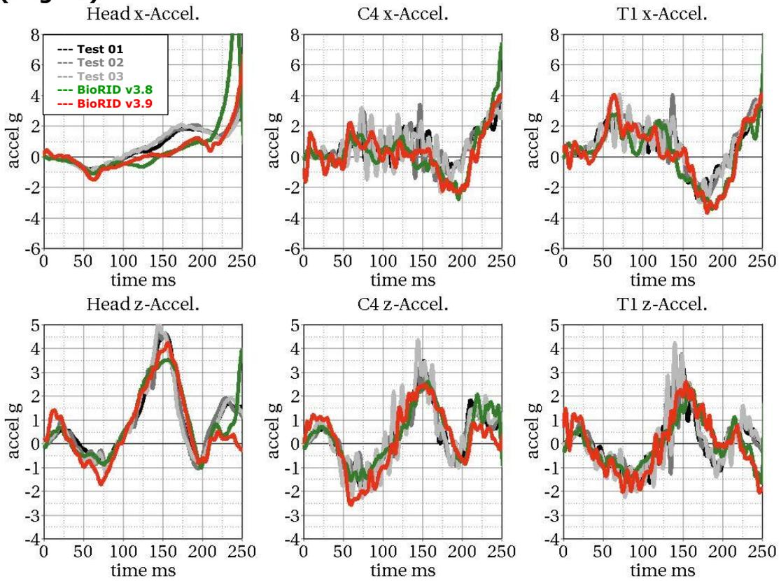
**Spine fixed up to L6 with damper/with muscle substitute springs
