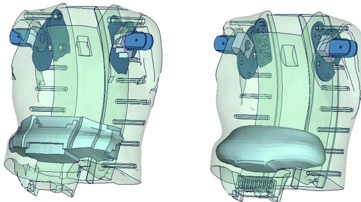
**Figure 17:** new mesh of the water cavity
