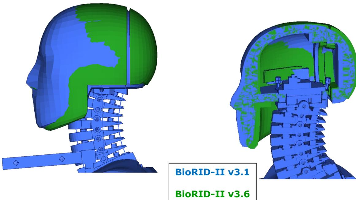
**Figure 13:** Head geometry of BioRID-II v3.1 compared to v3.6
