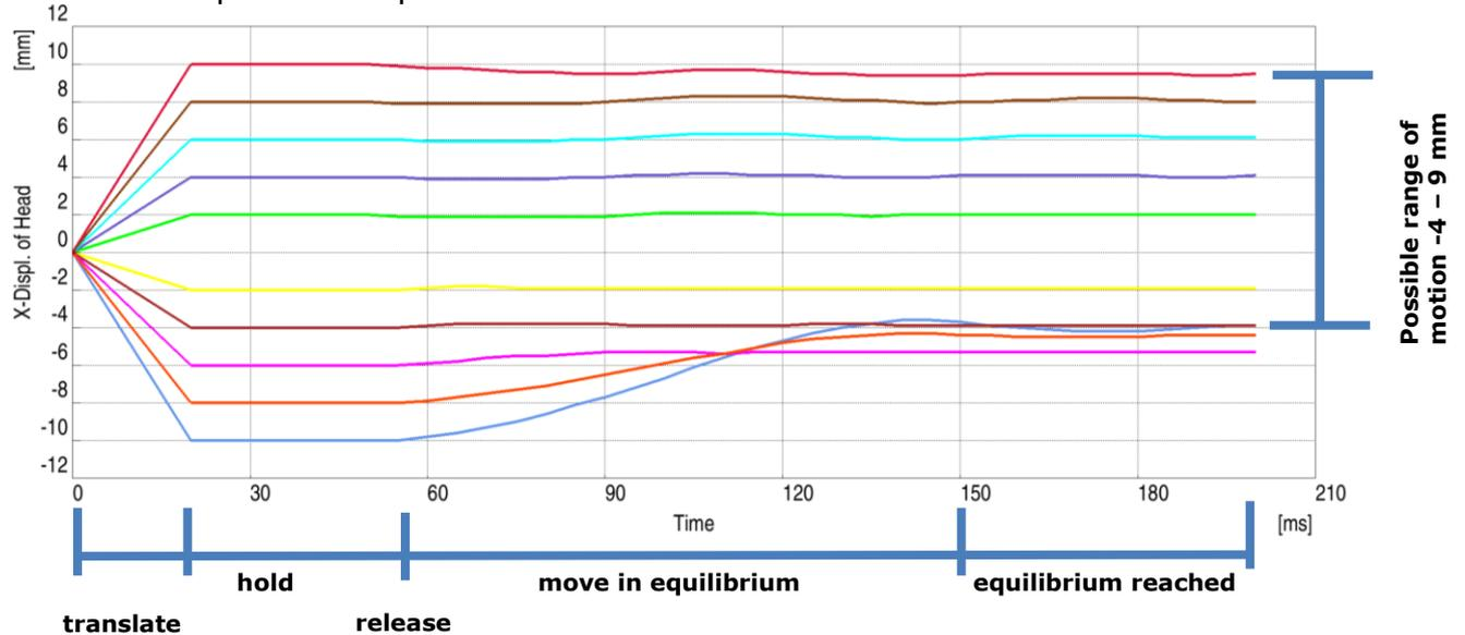
The curves show different phases of Head movement. At the end a possible range of motion is about 4mm forward and 9mm backwards.
