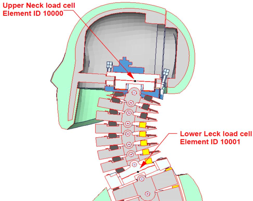
**Figure 5:** Model of lower and upper neck load cell
