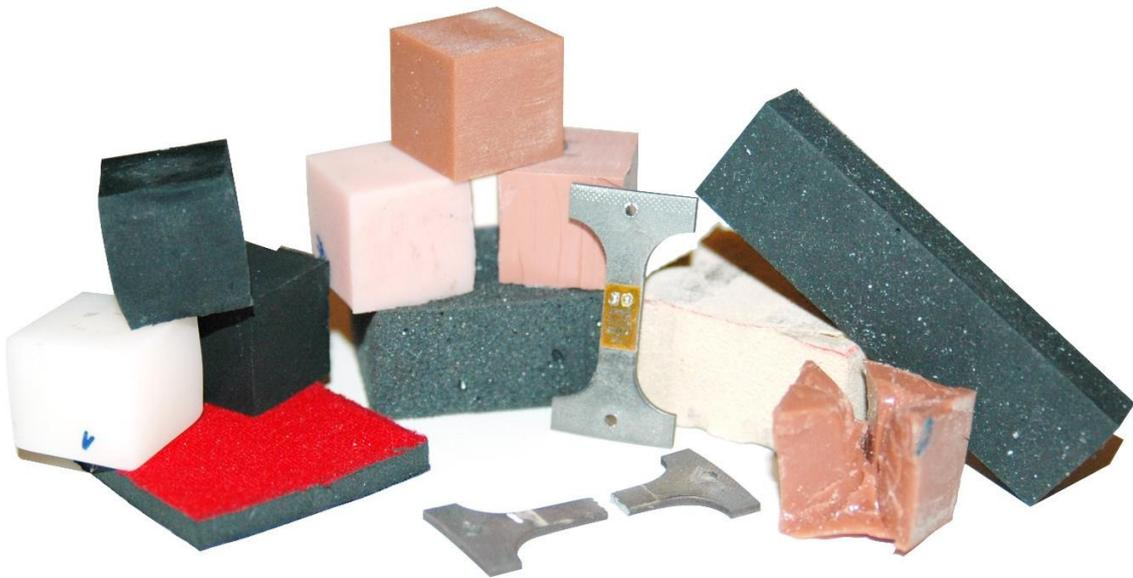
**Figure 30:** Material test samples of WorldSID
