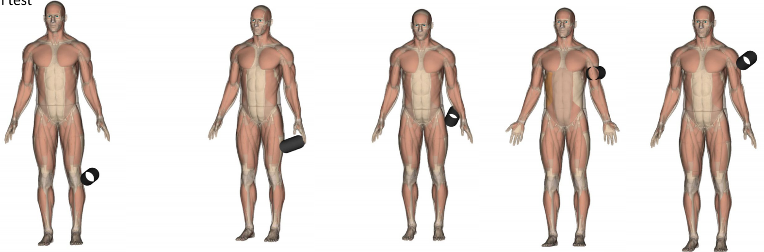
impactor tests with constant velocity ( v=30\text{kph} )
